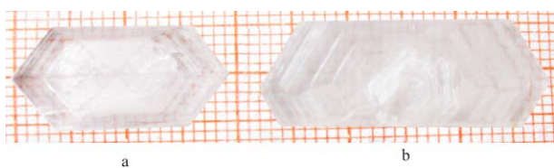
Fig. 1 Photographs of a – pure TTCC and b – Co 2+ -doped TTCC
